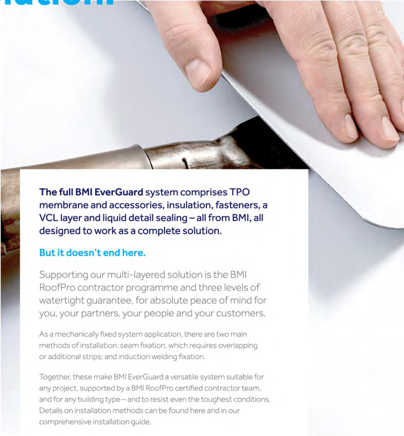
**The full BMI EverGuard system comprises TPO membrane and accessories, insulation, fasteners, a VCL layer and liquid detail sealing – all from BMI, all designed to work as a complete solution.**
